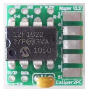
After the components are soldered, cut the components' leads with a wire cutter.
