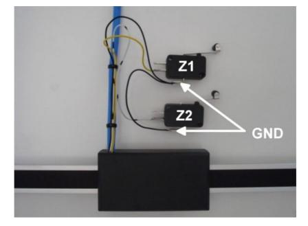
The black GND cable is connected to both switches.
