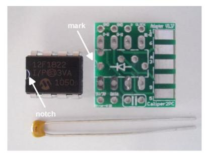
Double check that the IC is mounted in the right direction before the device is soldered (notice the notch and the mark on the PCB).
