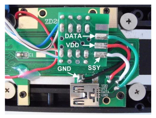
Secure the adapter on the encoder PCB with hot glue or with epoxy adhesive.
