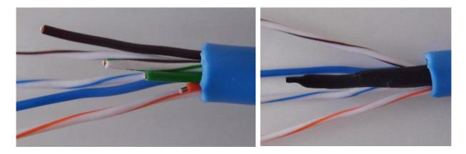
Solder the 4 wires of the patch cable to the 21BIT adapter according to the pin assignment.
