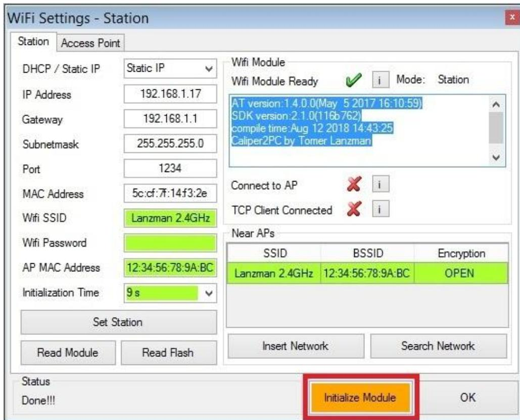
Close the Caliper2PC software and then restart it. The Caliper2PC interface is now configured as a station and can be connected to the host via your Wifi network.
