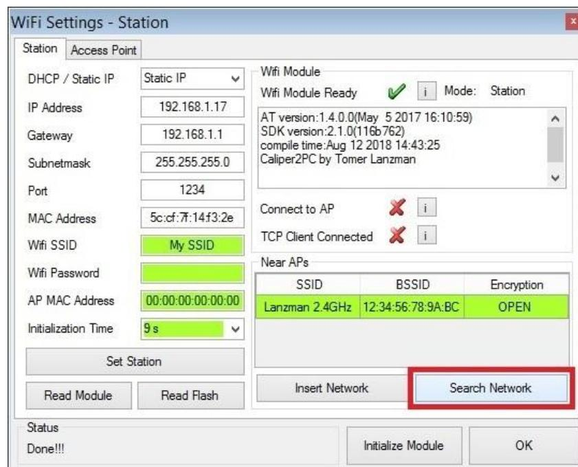
Select your Wifi network from the "Near APs" table and then click the "Insert Network" button to insert the Wifi SSID and the AP MAC Address (BSSID) into the green input fields.
