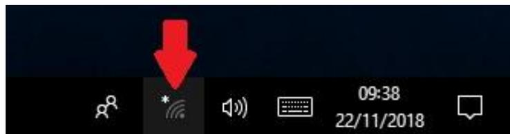
This opens the network panel displaying all available Wifi networks nearby. Select the Caliper2PC interface's Wifi network "Caliper2PC" ("Wifi SSID as defined in the settings) and click "Connect".
