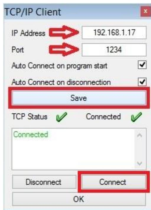
Please enter the IP address of the Caliper2PC interface (for example 192.168.1.17 see page 16) in the "TCP / IP Client" window's "IP Address" field. In the "Port" field, enter the port number defined in the interface (for example, 1234 see page 16). Then click the "Save" button to apply the values. Click on the "Connect" button to connect the TCP / IP client to the Caliper2PC interface.
