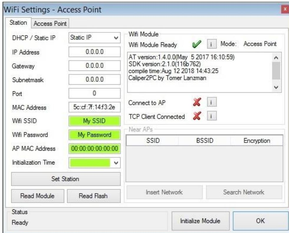
The appropriate IP address, subnet mask and gateway for the existing network can be taken from a local computer connected to the network. Please press the key combination "Windows (⊞)" + "R" and type the command "cmd" into the "Open" line of the "Run" window. Click the "OK" button to open a Command Prompt window.
