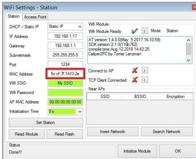
Please set the "Initialization Time" to 9 seconds. This is the time the interface will try to connect via Wifi before the USB interface is activated. The initialization time depends on the respective router or access point. The selected 9 seconds should be sufficient for most devices. All values used in this example are shown in the following table:
