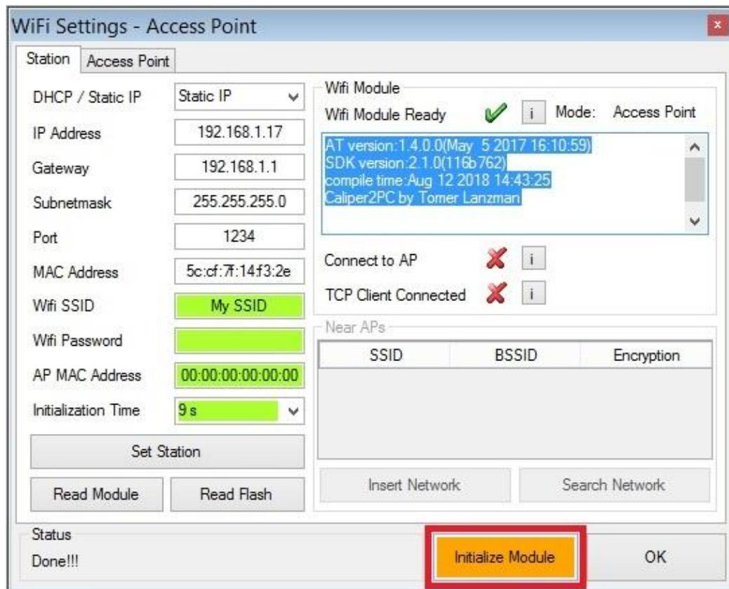
After the Caliper2PC software has been restarted, open the "WiFi Settings" window and wait until the status is set to "Done!!!". Click the "Read Flash" button so that the software will fill the input masks with the values from the flash memory.
