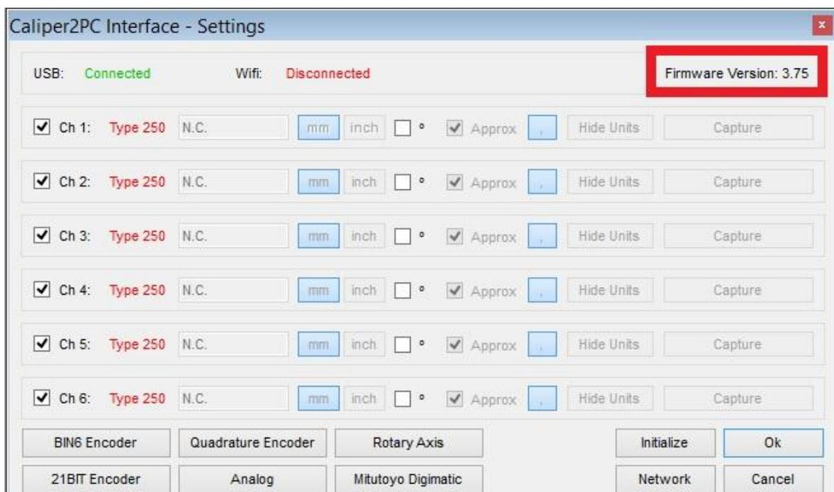
If the interface supports Wifi, it can now be configured as an access point or as a station. If the firmware version of the interface is before 3.75 Wifi is not supported. Upgrading interface versions prior to 3.75 to Wifi is not possible.
