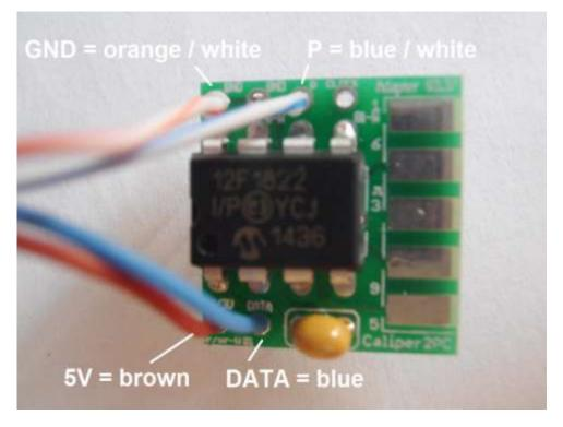
The connection of the analog adapter on the Caliper2PC interface side is now ready. Before carrying out the following steps, it is necessary to choose in which mode the analog adapter should run. Depending on the configuration of the MS1 and MS2 terminals (see below), the desired mode can be selected.
