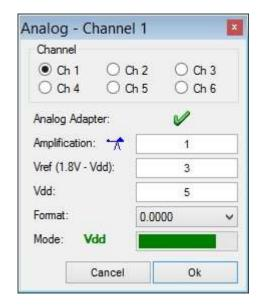
In the "Analog" window select the channel with the connected analog adapter (eg. channel 1). If an analog adapter was found at port "P1" during initialization, a green "V" appears on the "Analog" window.
