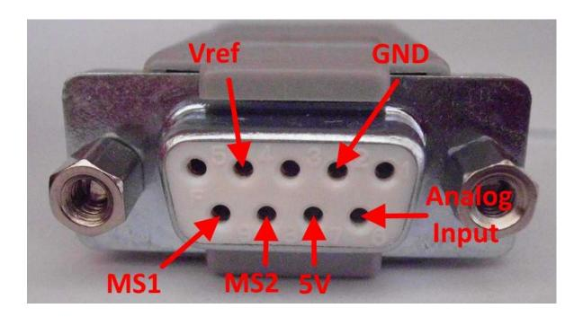
If the adapter PCB is installed in a 9-pin D-Sub connector, the pin assignment for the socket is:
