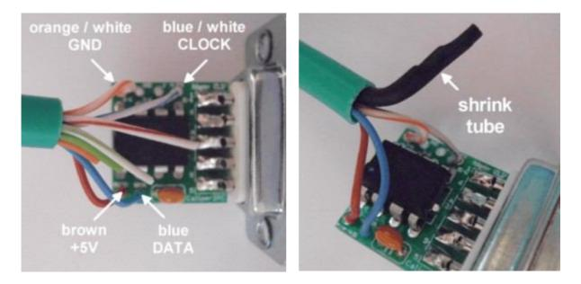
Solder the 4 wires of the patch cable to the quadrature adapter according to the pin assignment.
