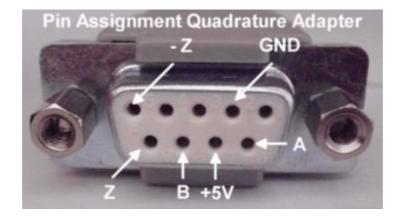
Important! If pin 4 is connected inside your glass scale's connector, pin 4 must be disconnected on the adapter PCB.
