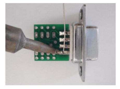
First, the PCB has to be soldered to the 9 pin D-SUB connector.
