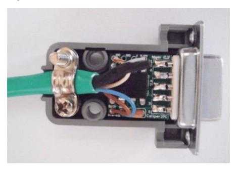
Lay the connector screws with the washers in the right position before closing the cage.
