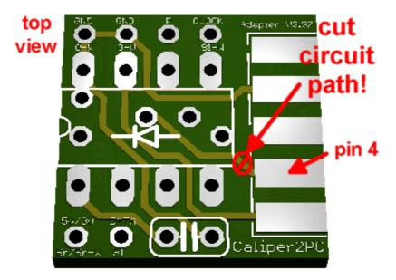
The circuit path can be cut with a carpet cutter or with a small Dremel grinder. Alternatively, the circuit path for disconnecting pin 4 can be cut on the bottom side of the PCB.
