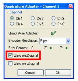
You have to know the approximate position of the reference mark you want to use to auto zero the axis. The Caliper2PC software will capture the precise position of the reference mark while the axis is driven in low speed through the reference mark's area. The green square "Z-LED" will turn red as soon as the reference mark
