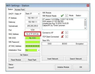
Please set the "Initialization Time" to 9 seconds. This is the time the interface will try to connect via Wifi before the USB interface is activated. The initialization time depends on the respective router or access point. The selected 9 seconds should be sufficient for most devices. All values used in this example are shown in the following table:
