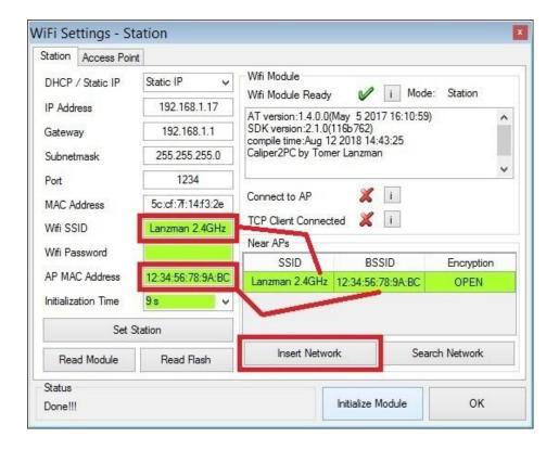
If your Wifi network is not encrypted, leave the input field "Wifi Password" empty. If your Wifi network is encrypted, enter the Wifi password into the input field. Click the "Set Station" button to write the values to the flash memory. After the status has been set to "Done!!!", click the "Initialize Module" button that appears in orange color.
