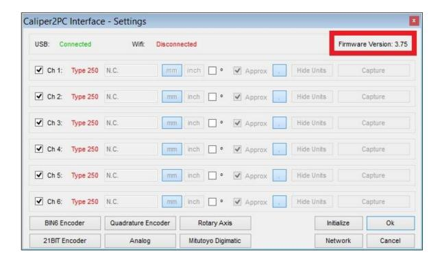
If the interface supports Wifi, it can now be configured as an access point or as a station. If the firmware version of the interface is before 3.75 Wifi is not supported. Upgrading interface versions prior to 3.75 to Wifi is not possible.
