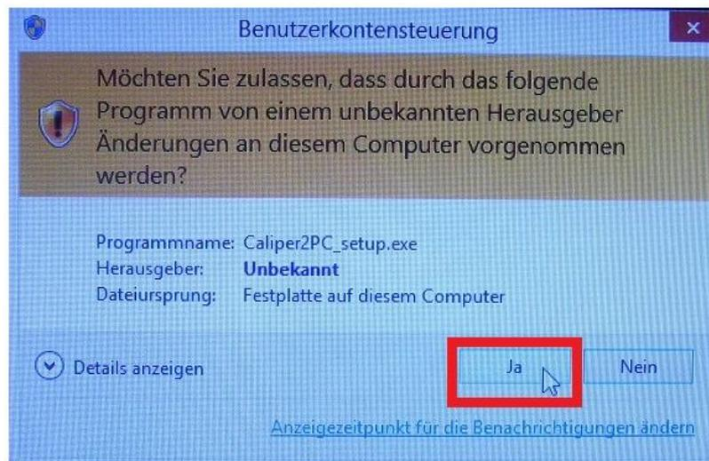
Confirm the next message and allow the Caliper2PC software to be installed.
